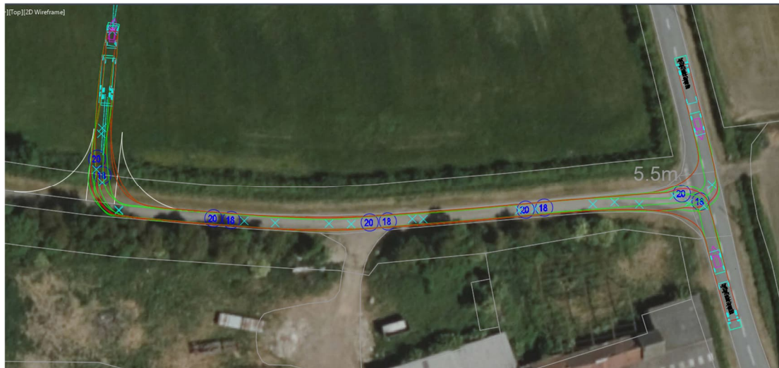
Plate 2-11: Brick Kiln Lane and Trumfleet Lane Junction Tractor and Trailer 10.0 m SPA
