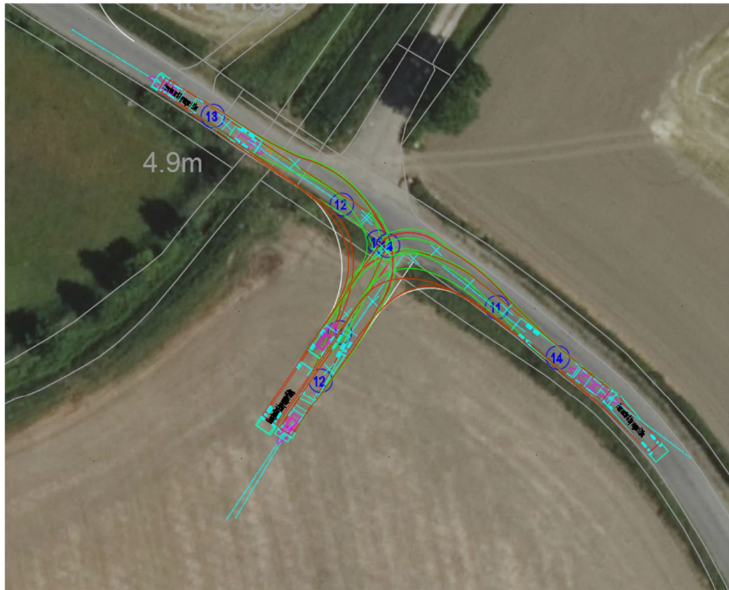
Plate 2-16: South off Marsh Road Swept Path Analysis Tractor and 12.0 m Trailer
