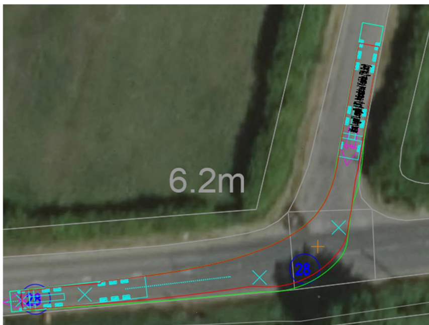
Plate 2-11: SPA Southbound Turning Right onto Moss Road Max Legal HGV No Junction Improvement Works
