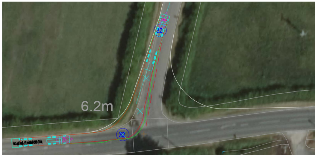
Plate 2-13: SPA Eastbound Turning Left onto Fenwick Common Lane Max Legal HGV with Junction Improvement Works
