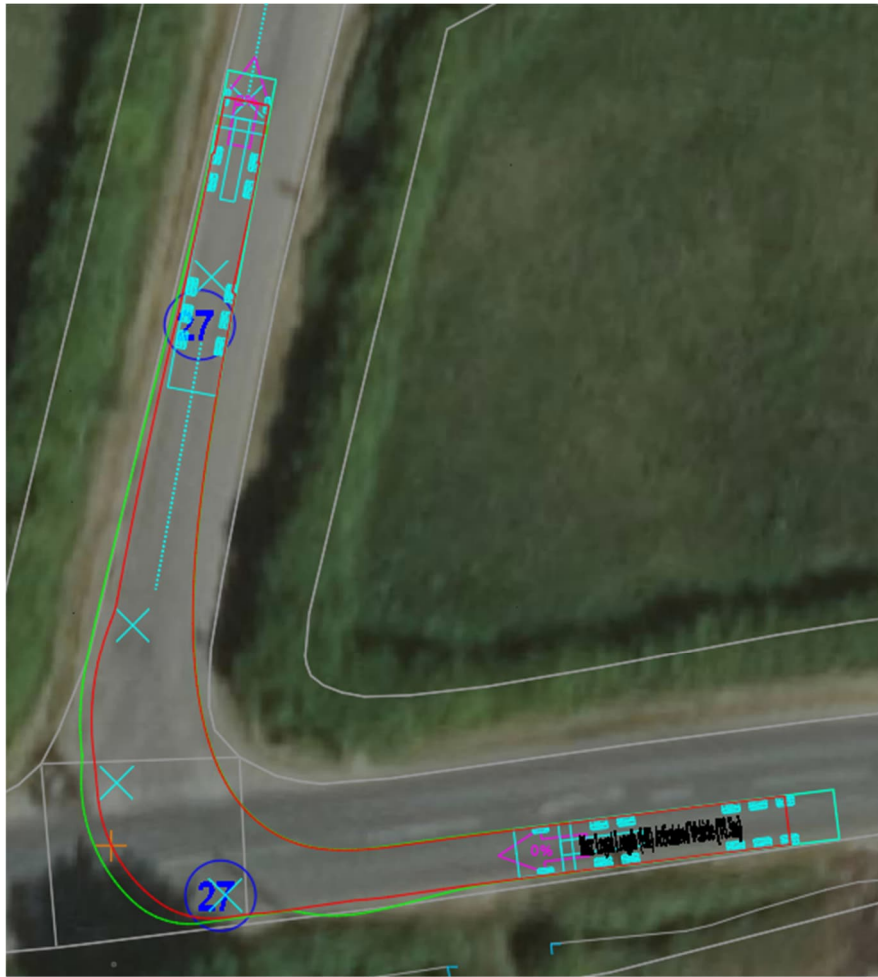
Plate 2-10: SPA Westbound Turning Right onto Fenwick Common Lane Max Legal HGV No Junction Improvement Works
